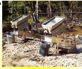
A sluice with running water from a tank on the top pushes the lighter dirt down and out the bottom while gold pieces and flake remain in the sluice for collecting.
