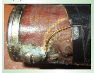
The photo shows my 160m resonator that became intermittent after 2 years on the roof. After peeling back the outer insulation it was revealed that the connection was covered in a crispy crud of corrosion. Thankfully I was able to break it down, clean up the wires and termination screw and washers, and put things back to rights. A good application of waterproof grease on the screw and wires and a few layers of good old "Scotch-88" finished up the patch job for another couple of years.
